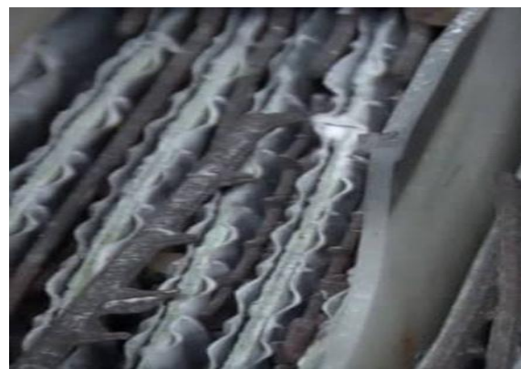
Figure 2 Sulphated Battery Cells [1]
