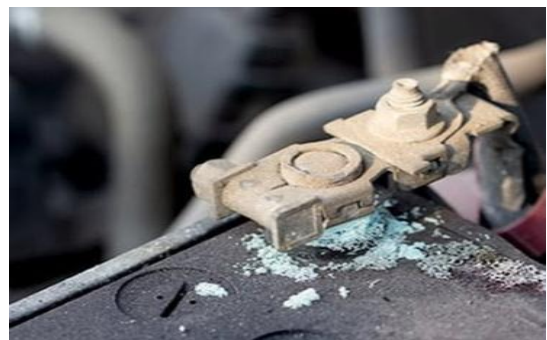
Figure 1 Sulfated Battery Terminals [1]
