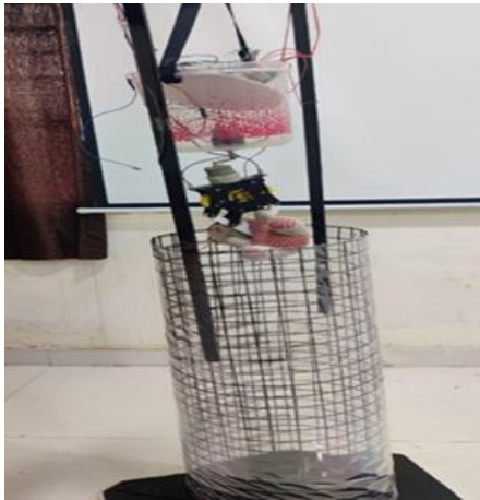
Figure 9 Child Rescue Demonstrating Victim Pick-Up Mechanism
