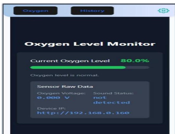
Figure 1 Monitoring Dashboard: The Interface Displays Real-Time Oxygen Levels and Sound Activity, Helping Users Monitor Child Safety Conditions Inside the Vehicle
