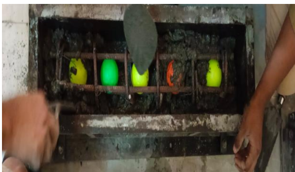
Figure 2 Casting of the Beam Specimen
