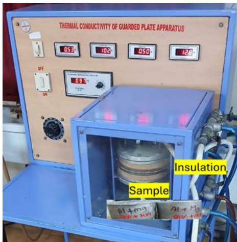
Figure 1 Experiment Setup for Thermal Conductivity Measurement
