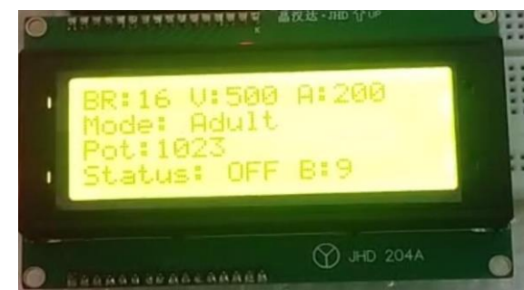
Figure 6 The Adult Mode is Enabled with a Breath Rate of 16
