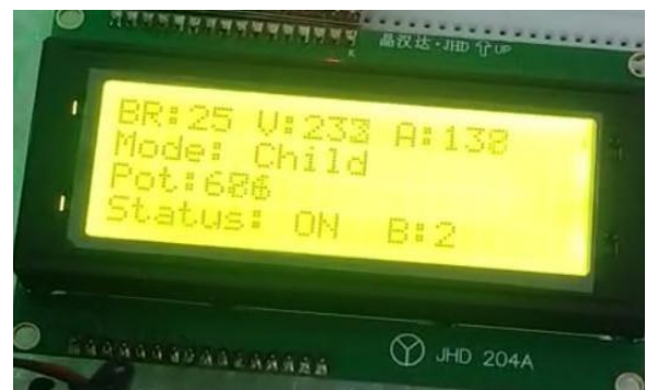
Figure 5 The Child Mode is Enabled with a Breath Rate of 25
