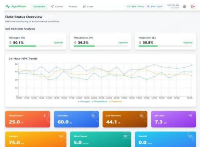
Figure 9 Dashboard to Monitor Soil Trends Over Various Parameters
