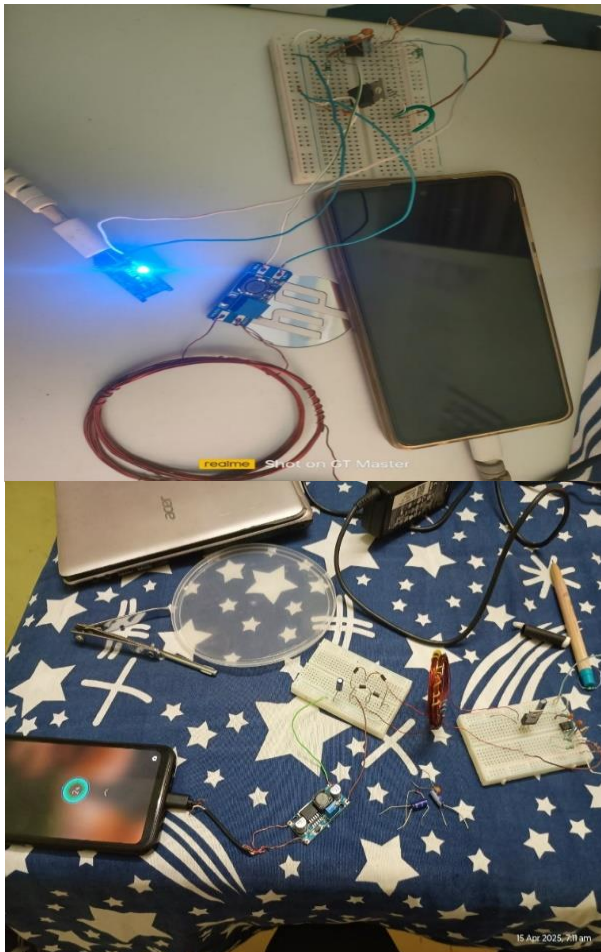
Figure 4 Represents Charging of Mobile at Supply Of 5V – 2.5A Rating
