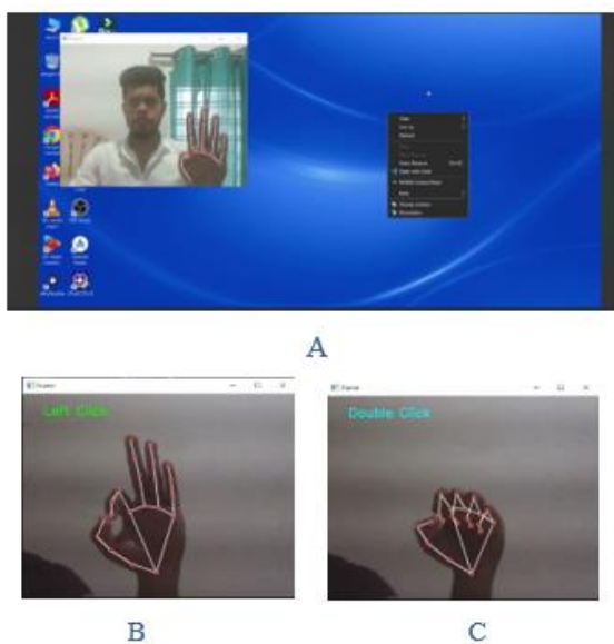
Figure 3 Visual Output of Hand Gesture-Based Mouse Control
