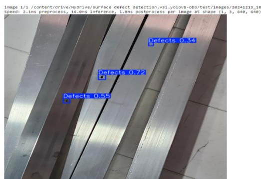
Figure 3 Output1 of Defects in Aluminium Surfaces
