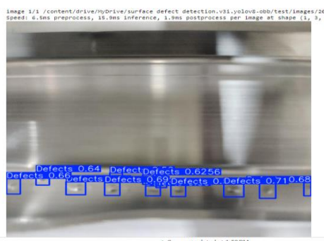
Figure 4 Output2 of Defects in Aluminium Surfaces
