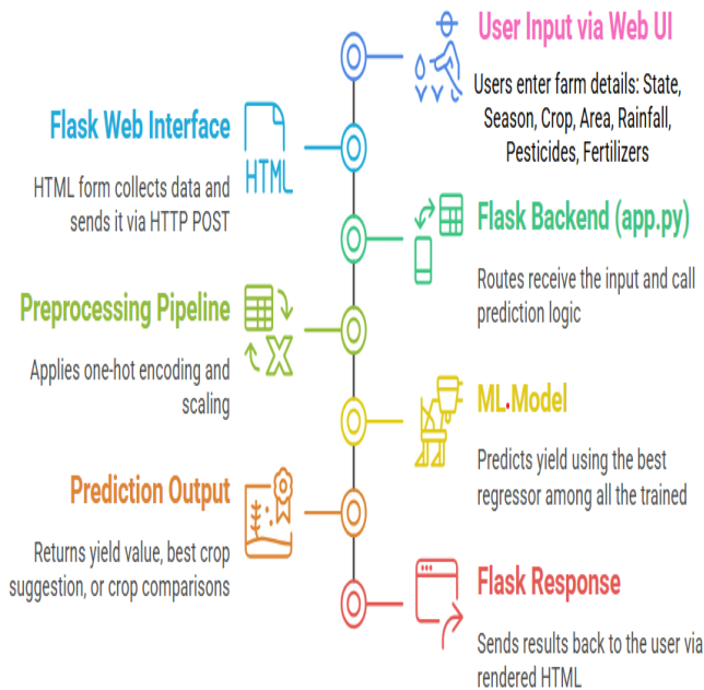
Figure 1 System Architecture for Agriculture Data Analysis and Crop Yield Prediction using Machine Learning
