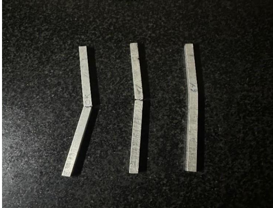
Figure 11 3-Point Bending Test Specimens After Failure
