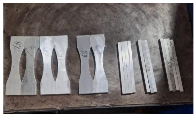
Figure 5 Fatigue and Flexural Specimen ASTM
