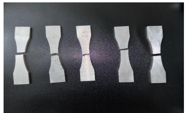
Figure 6 Fatigue Test Specimens After Failure
