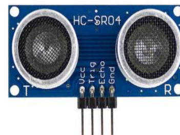
Figure 5 Ultrasonic Sensor HC-SR04
