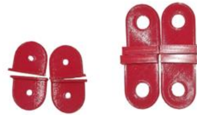
Figure 2 Shows 3d Printed Components of Motor Brackets
