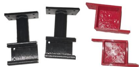
Figure 3 Shows 3d printed Components of Motor Mounting
