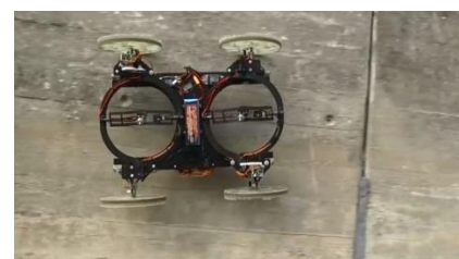
Figure 9 Shows Final Assembly of Wall Climbing Robot
