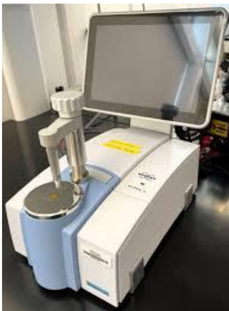
Figure 5 FTIR Spectroscopy Identify Plastics
