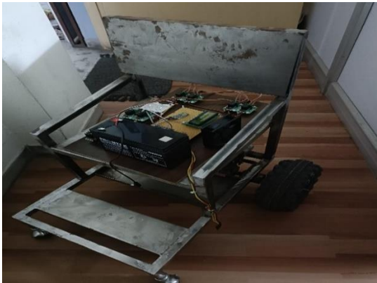
Figure 6 Hardware Model of Solar Powered Gesture Controlled Wheel Chair with Integrated Home Automation Using Convolutional Neural Network
