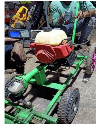
Figure 34 Machine Under Test with E-Glass Fibre Composite Leaf Spring
