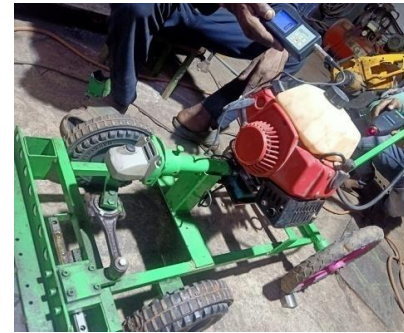
Figure 30 Machine Under Test with Conventional Rubber Mount
