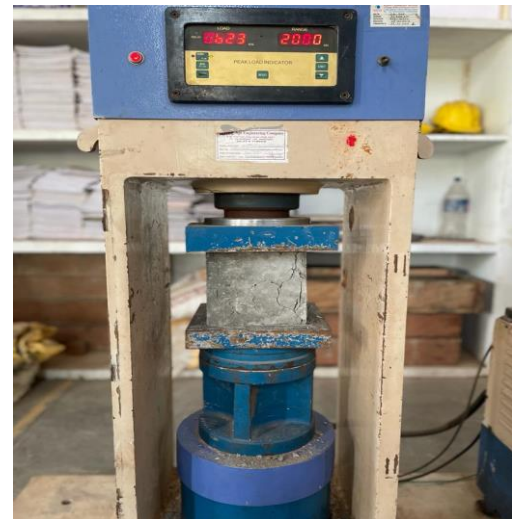
Figure 1 Cube Compressive Strength Testing Machine
