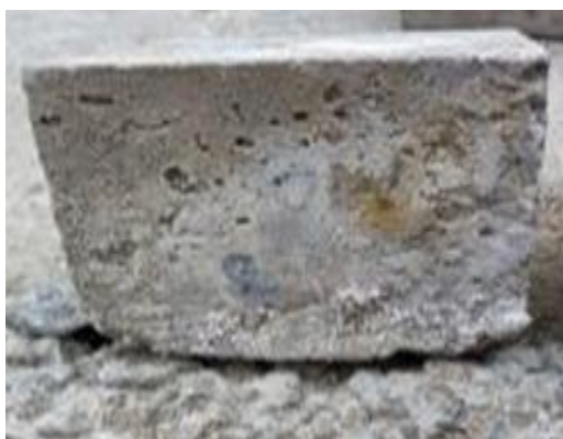
Figure 4 Visual Inspection of Cube Specimen Subjected to H_2SO_4 Acid Attack After 28 Days
