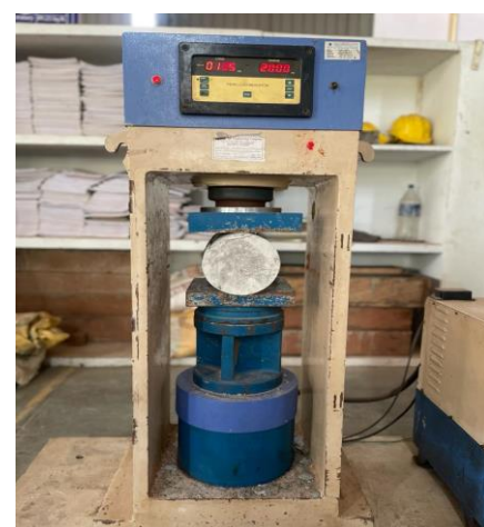
Figure 2 Cylinder Splitting Tensile Strength Testing Equipment
