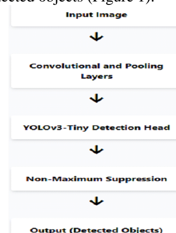
Figure 1 YOLOv3-Tiny Detection Flow
