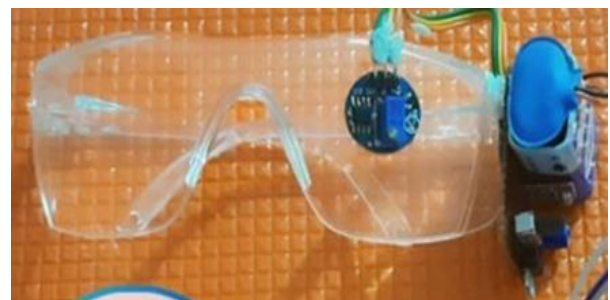
Figure 7 Driver Drowsiness Detection System in order to Avoid Accidents Device
