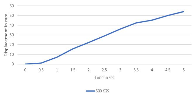
**Graph 5** Displacement of High Strength Steel Wind Turbine Subjected to Blast Loading at The Top
