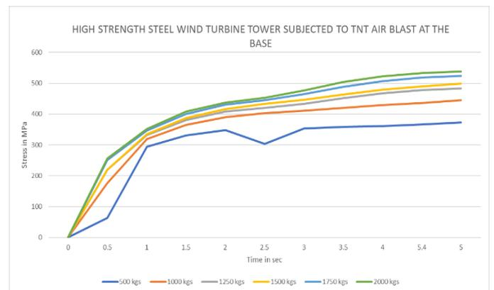
**Graph 1 Von Mises Stress of High Strength Steel Wind Turbine Subjected to Blast Loading at The Base of the Tower**
