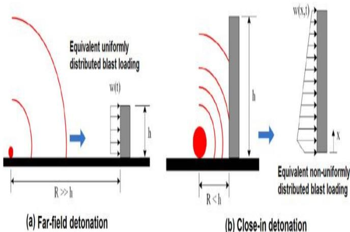
**Figure 1 Representation of Blast Load Detonation Acting on the Structure**
