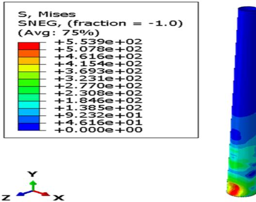
**Figure 8 Simulation of High Strength Steel Turbine Tower Subjected to 1750 Kgs Blast Load At the Base**
