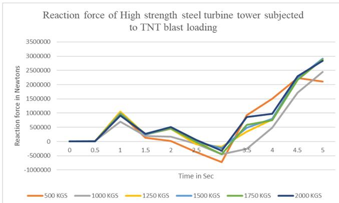
**Graph 3** Reaction Force of High Strength Steel Wind Turbine Subjected to Blast Loading at The Base
