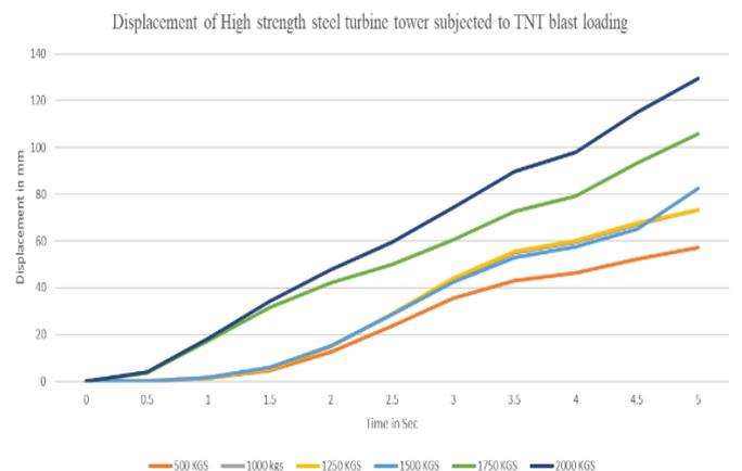
**Graph 2 Displacement of High Strength Steel Wind Turbine Subjected to Blast Loading at The Base of the Tower**
