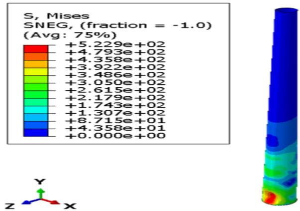
**Figure 7 Simulation of High Strength Steel Turbine Tower Subjected to 1500 Kgs Blast Load At the Base**
