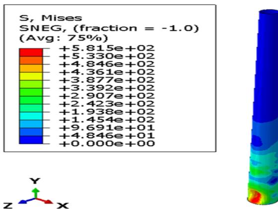
**Figure 9 Simulation of High Strength Steel Turbine Tower Subjected to 2000 Kgs Blast Load At the Base**
