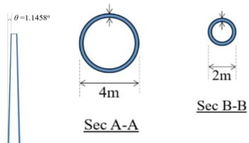
**Figure 3** Geometric Dimension of the Wind Turbine Tower
