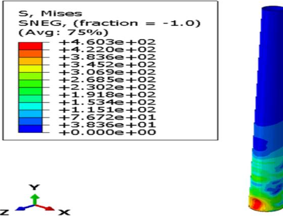
**Figure 5 Simulation of High Strength Steel Turbine Tower Subjected to 1000kgs Blast Load At the Base**
