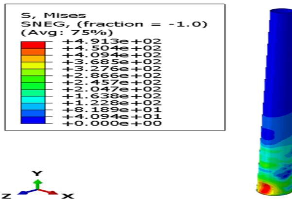
**Figure 6 Simulation of High Strength Steel Turbine Tower Subjected to 1250 Kgs Blast Load At the Base**
