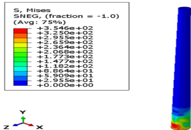
**Figure 4 Simulation of High Strength Steel Turbine Tower Subjected to 500kgs Blast Load At the Base**
