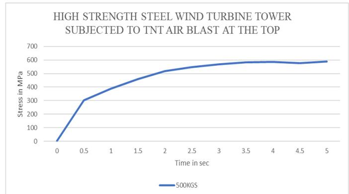
**Graph 4** Von Mises Stress of High Strength Steel Wind Turbine Subjected to Blast Loading at The Top
