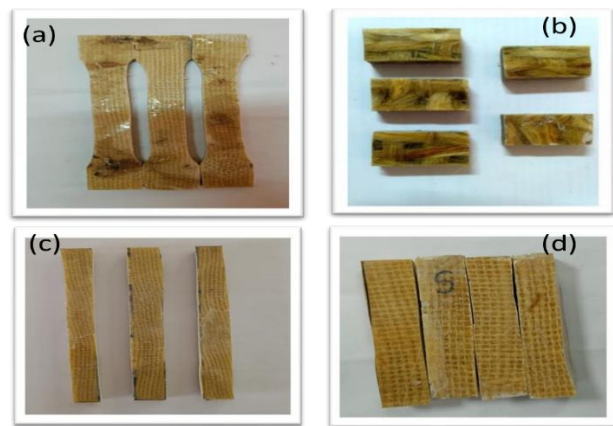
Figure 2 Test Specimen (a) Tensile (b) Compression (c) Flexural (d) Impact (e) Sisal Roselle/Epoxy Hybrid polymer composite Specimen Under Tensile Test, f) Composite Under Compression Test, g) Flexural Sample Under Test, h) Impact Sample Under Test
