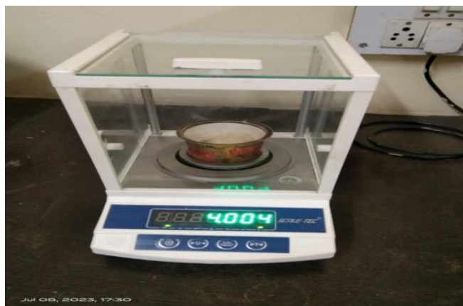
Figure 5 Weight of the Powder Taken with The Help of Weighing Scale
