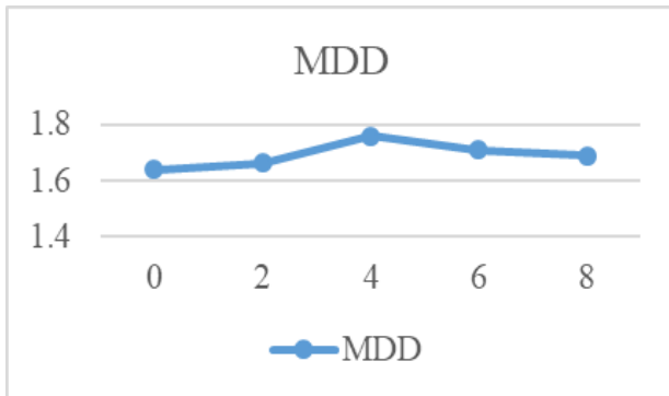
Figure 5 Plot between Percentage of Lignin and Maximum Dry Density
