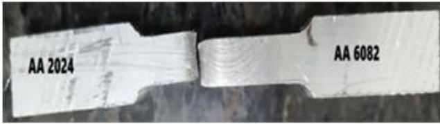
Figure 5 Tensile Specimen After Failure
