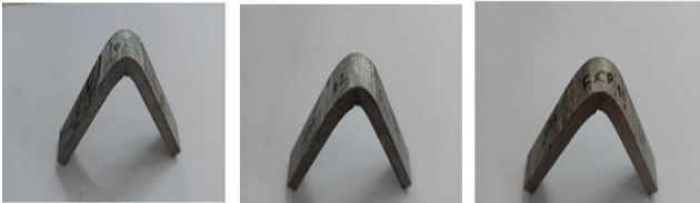
Figure 6 Specimen After Bending
