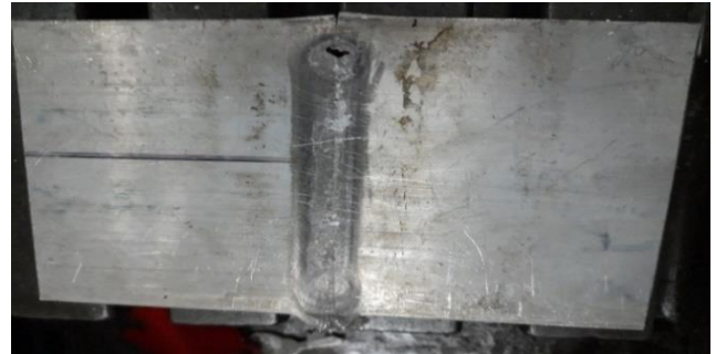
Figure 3 After Friction Stir Welding Plate
