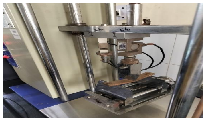
Figure 4 Specimen Fracture During Flexural Test
