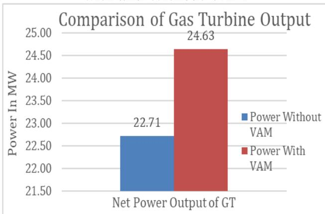
The total net power output is increased by about 1.86 MW; the same is represented in the graphical form as shown in figure 5.
