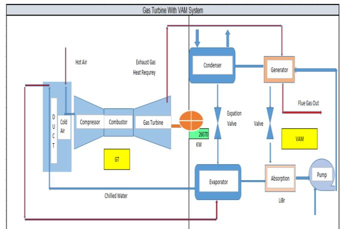
**Figure 4 Schematic Diagram of the VAM Installation in FG Duct with Gas Turbine Air Intake System**
