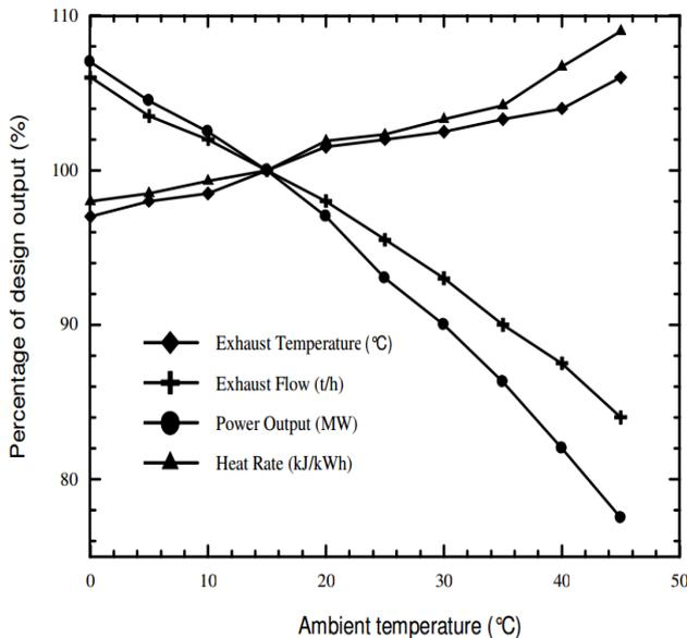
**Figure 2 Effect of Ambient Temperature On Gas Turbine Performance**
