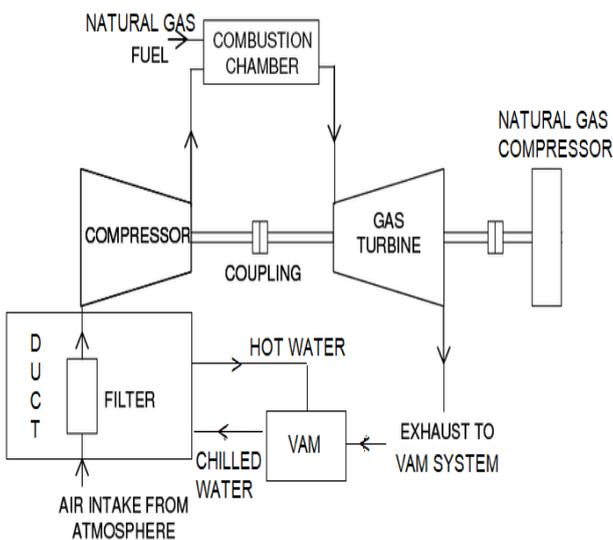
**Figure 3** GT Block Diagram with Proposed Modification
