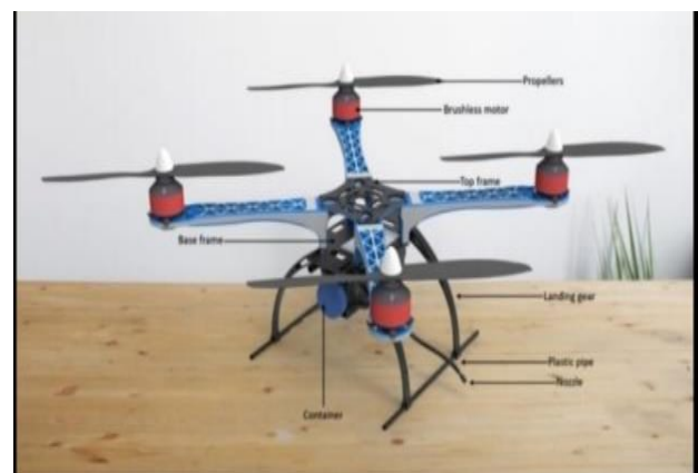
Figure 15 SolidWorks Model of Agricultural Quadcopter with Spraying Mechanism
