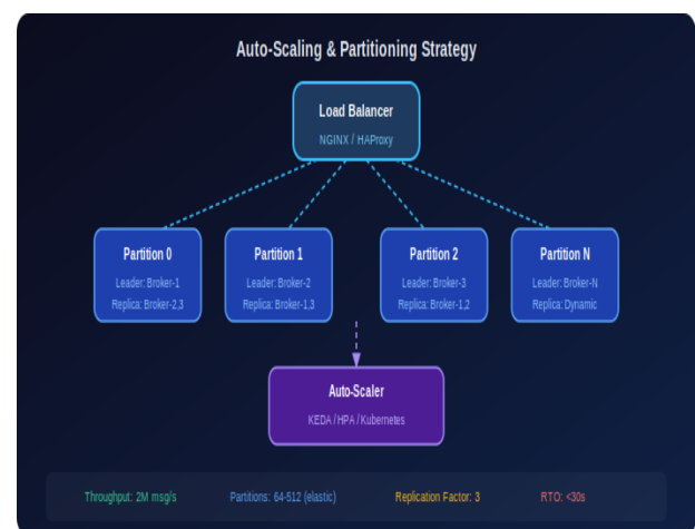
Figure 4 Partition topology and auto-scaling strategy: Kubernetes-based elastic scaling triggered by consumer lag and CPU metrics.
