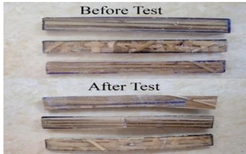
Figure 6 Composite Specimens Before and After Flexural Testing
