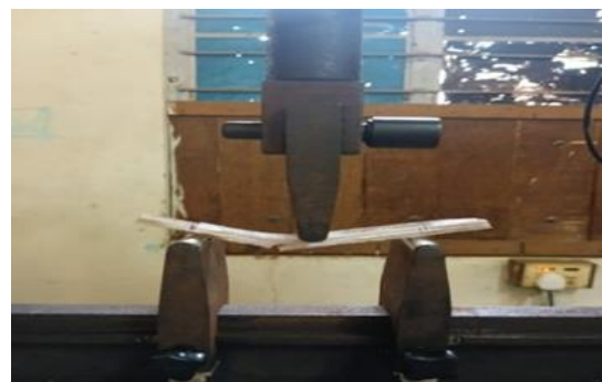
Figure 5 Composite Specimen Mounted for Three-Point Bending Test
