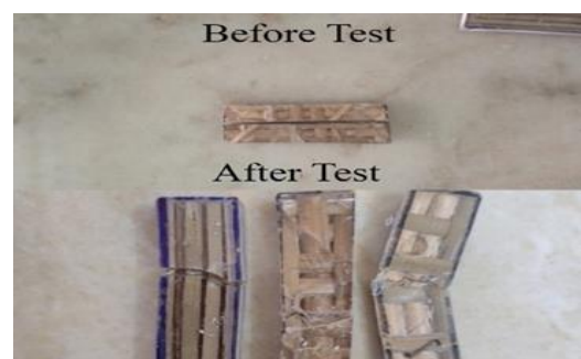
Figure 2 Tensile Test Specimens Before and After Failure
