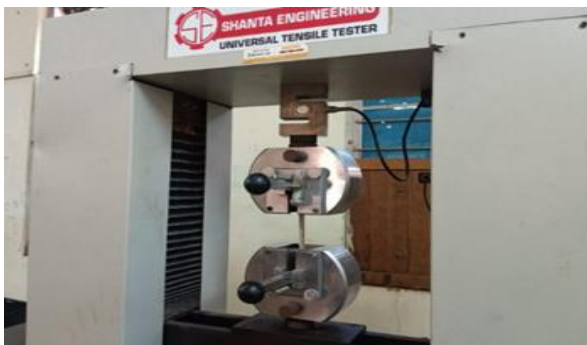
Figure 3 Gripping Arrangement of the Test Specimen in the Universal Testing Machine
