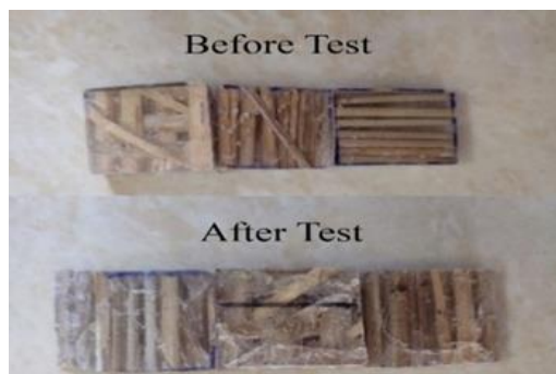
Figure 7 Flexural Failure of Composite Specimens
