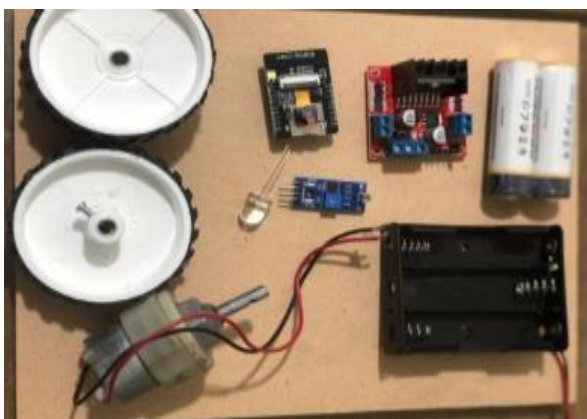
Figure 2 Disassembled view of all hardware components used in the prototype
