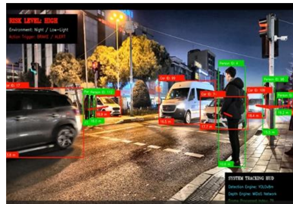
Figure 2 Real-time visual inference snapshot displaying multi-object bounding box tracking, MiDaS-driven depth distance estimation (meters), and proactive kinematic threat state calculation under clear environmental testing conditions
