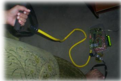
Figure 6 Real time exercise monitoring without ZigBee module
