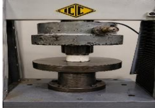
Figure 11 Compression test for PLA+PBS Sandwich material
