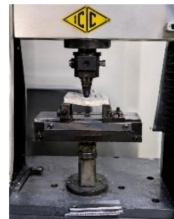
Figure 10 flexural test for PLA+PBS sandwich material
