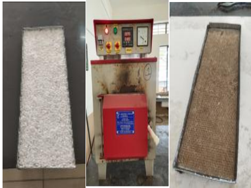
Figure 8 Heating and melting process of PBS
