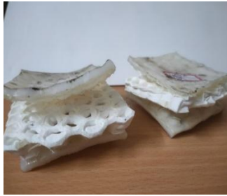
Figure 15 compression Tested Specimens
