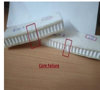
Figure 13 Flexural tested Specimens
