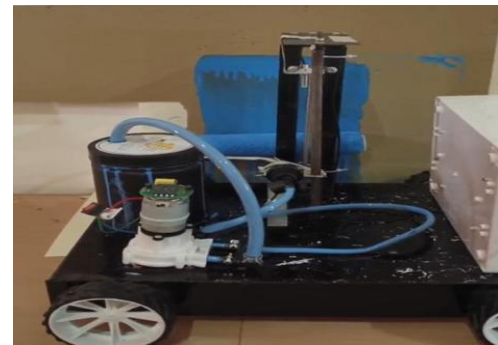
Figure 3 Physical prototype of the PLC-based automated roller wall painting system showcasing integrated pump, roller mechanism, and control unit
