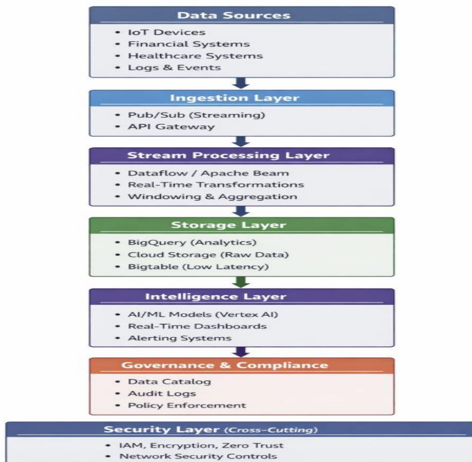
Figure 1 High-Level Block Diagram of the Proposed Architecture
