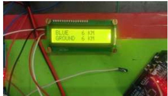
Figure 5 Distance Estimation of the Faults
