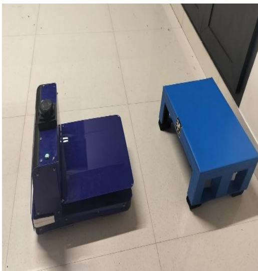
Figure 5 Pre-Engagement Position Of The Robot With Pallet
