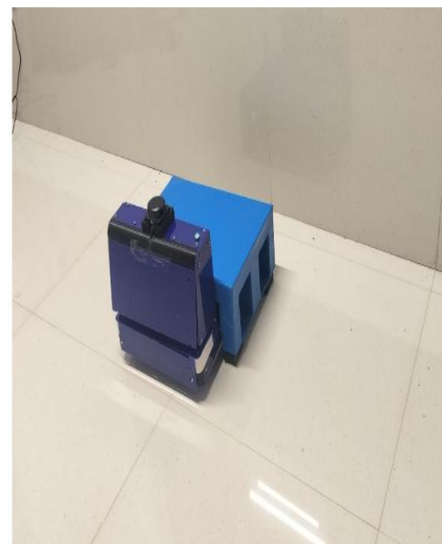
Figure 6 Fully Inserted And Lift-Ready Position
