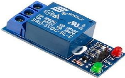
Figure 6 Module for Relays
