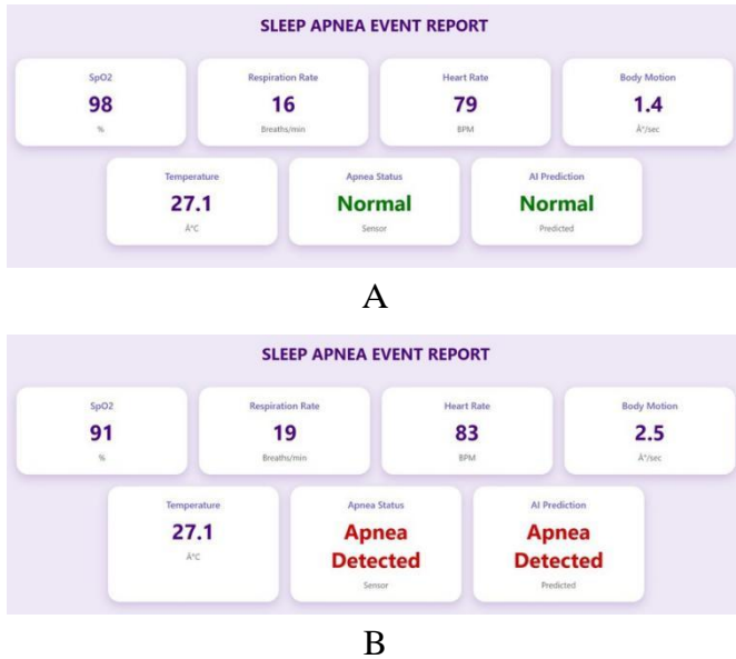
Figure 3 Software output of the system showing (A) normal sleep monitoring and (B) apnea detection.
