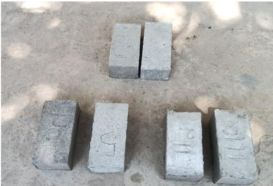
Figure 8 Prepared Concrete Test Specimens (Bricks/Blocks) for Compressive Strength Evaluation
