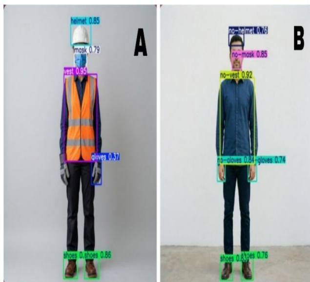
Figure 3 Yolov11-Based Real-Time Ppe Detection Output Showing (A) Compliant Worker And (B) Non-Compliant Worker With Confidence Scores For Each Detected Class.
