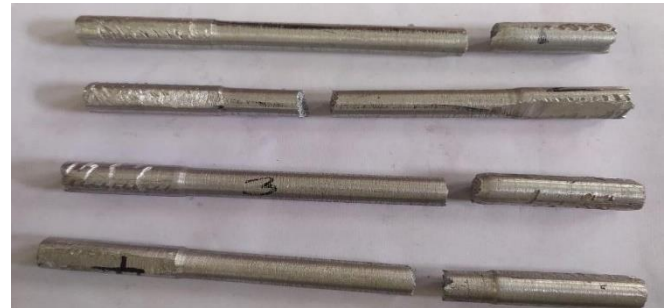
Figure 12 After Tensile Test of the Specimen
