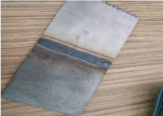
Figure 1 TIG Welding Through Using Dissimilar Metal SS409 & ASS304
