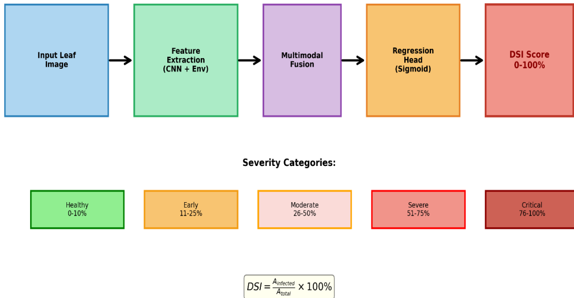
Figure 4. Disease severity estimation workflow showing the progression from input image through feature extraction, fusion, regression head, to DSI score with categorical severity thresholds (Healthy 0-10%, Early 11-25%, Moderate 26-50%, Severe 51-75%, Critical 76-100%).
