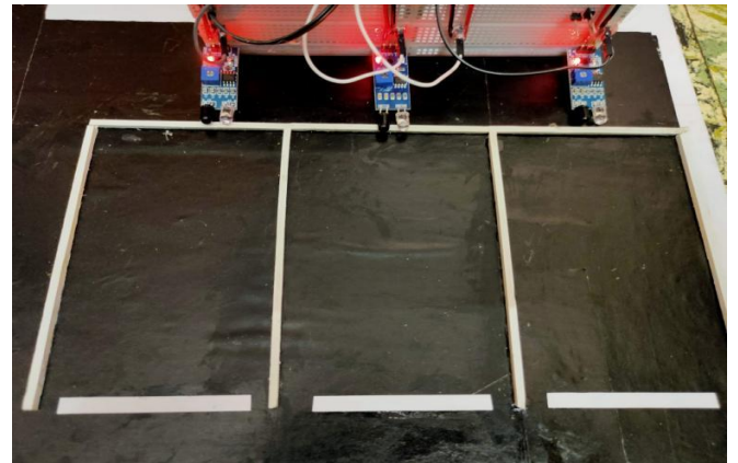
Figure 4 Parking Slot with IR Sensors
