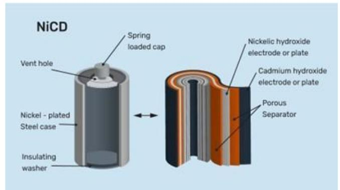
**Figure 2 Structure of Ni-Cd Battery**
