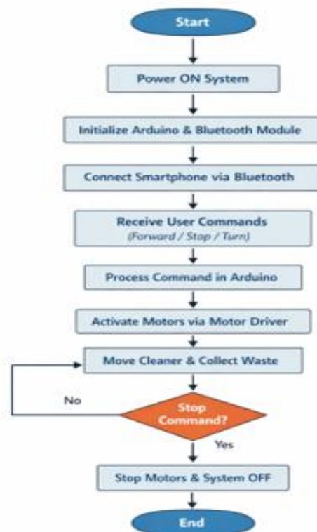
Flow Chart 1 Illustrates the Step-by-Step Operational Sequence of the Arduino-Based Bluetooth-Controlled Village Pond Cleaner
