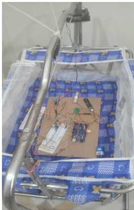
Figure 10(a) Internal Arduino Setup of the Cradle
