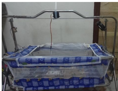
Figure 10(b) External Setup with Swing Mechanism
