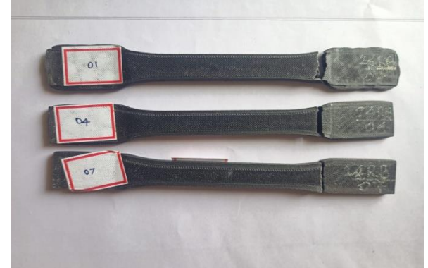
Figure 8 After Tensile Test of the Specimen
