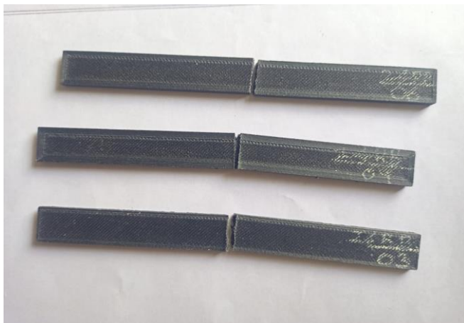
Figure 11 After Flexural Testing of the Specimen
